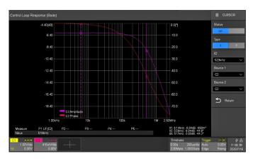
The oscilloscope can control the built-in waveform generator or a stand-alone Teledyne Test Tool generator, to scan the amplitude and phase-frequency response of the DUT, and display the data as a Bode Plot. This makes it possible to replace expensive network analyzers in some applications.
