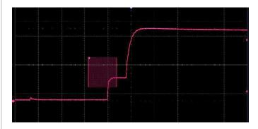
Trigger Zone is available for advanced triggering. Combine spatial triggering with common trigger mode to isolate signals of interest.
