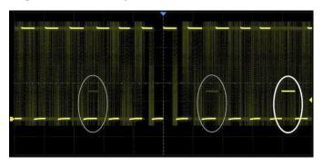
With a waveform update rate of up to 200,000 wfm/s, the oscilloscope can easily capture unusual or low probability events. In Sequence mode, the waveform capture rate can reach 890,000 wfm/s.
