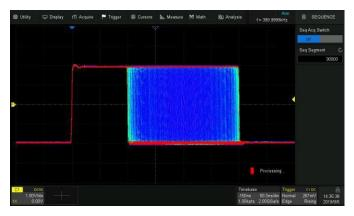
Segmented memory collection will store the waveform into multiple memory segments (up to 80,000) and each segment will store a triggered waveform as well the dead time information. The interval between segments can be as small as 2 µs. All of the segments can be played back using the History function.
