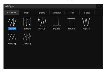
The 50 MHz waveform generator can output waveforms with up to 50 MHz frequency and  $\pm 3$  V amplitude. Six basic waveforms plus multiple types of arbitrary waveforms are built-in.
