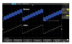
Enhanced Resolution (Eres) mode can improve the SNR without needing a repetitive waveform. Extra resolution bits can be added 0.5 bits at a time up to +3 bits.
