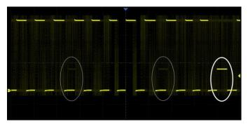
With a waveform update rate of up to 100,000 wfm/s, the oscilloscope can easily capture unusual or lowprobability events. In Sequence mode, the waveform capture rate can reach 500,000 wfm/s.
