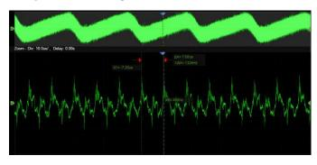
Using hardware-based Zoom technique and record length of up to 100 Mpts, users can select a slower time-base without compromising the sample rate, and then quickly zoom in to focus on the area of interest.
