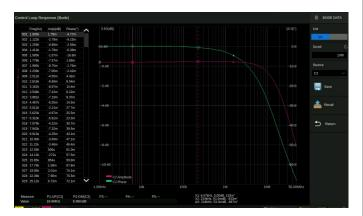
T3DSO1000HD can control the USB AWG module, control an independent Teledyne Test Tools T3AFG scan a devices amplitude and phase frequency response, and display the data as a Bode Plot. There is also a Vari-level Mode for accurately measuring Power Supply Control Loop Response (PSRR).
