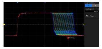
Segmented memory collection will store the waveform into multiple memory segments (up to 80,000) and each segment will store a triggered waveform as well the dead time information. The interval between segments can be as small as 2  $\mu$ s. All segments can be played back using the History function.
